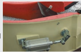
Pneumatically activated separation flap
